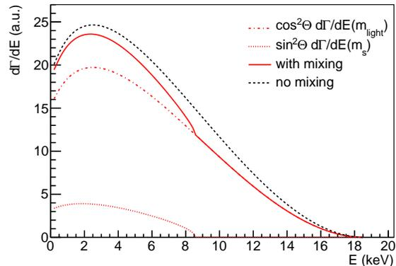
FIG. 1. Differential tritium  $\beta$ -decay spectrum without active-to-sterile neutrino mixing (black dashed line) and with mixing of a sterile neutrino with  $m_s = 10$  keV and  $\sin^2\theta = 0.2$  (red solid line). The red dashed lines depict the two components of the spectrum with active-to-sterile neutrino mixing.
