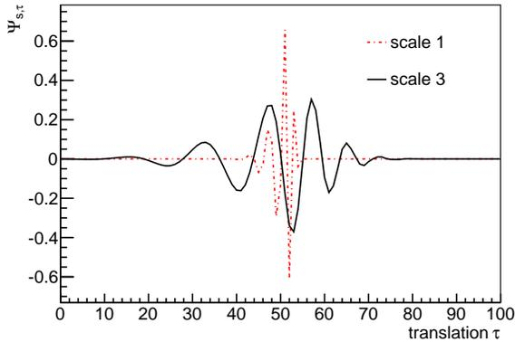
FIG. 3. Comparison of two different scales (1,3) of the mother wavelet *Daubechie 18*. The wavelet of scale 1 covers a rather large frequency range (see figure 2), is however very localized in  $\tau$ . Wavelets of larger scale cover smaller frequency ranges, but are less localized in  $\tau$ .
