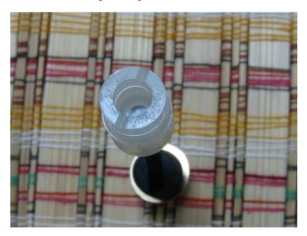
Anti Rotation slot, at the bottom of the connector:
