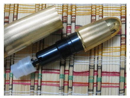
The filler unit requires the application of some type of a thread locker to retain it in the barrel. I used the rosin based section sealant from Tryphon. You may use currently available equivalents. I used a light coat of pure silicone oil on the piston seal for lubrication.
