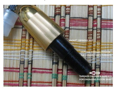
Filler assembled, ready to be re-fitted to barrel using the MB tool:
